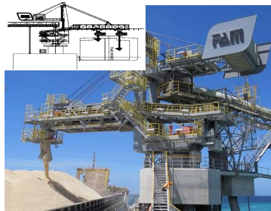
Project: Taiheiyō Engineering Corporation, Port Bohol, Limestone 1x SL 1200 tph, Philippines supplied by FAM Beumer Group
