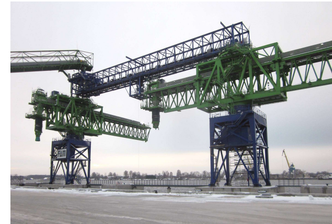
Project: LLC Riga Fertilizer, Terminal Riga, Latvia, twin SLs 1900 tph, urea, supplied by FAM Beumer Group
