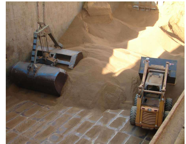
Example of cleaning hold with mobile equipment [Figure Wikimedia commons]
