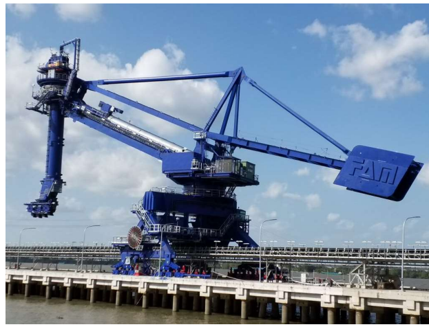
Project: 2 x CSUs 850 tph, coal, Power station Song Hau 1, Vietnam, supplied by FAM Beumer Group
