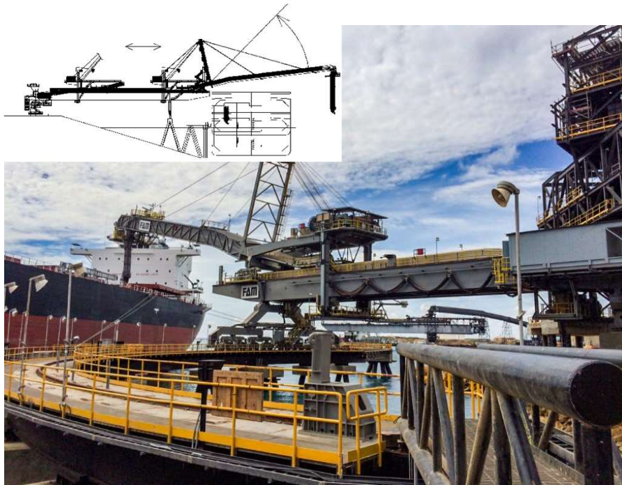
Project: Carbones del Cerrejon Ltd., Port Puerto Bolivar, 2 Quadrant SLs 6600 tph, supplied by FAM Beumer Group
