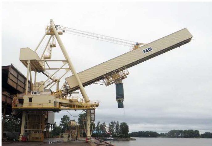
Project: East Europe, 3 x ship loaders 1500 tph, 60.000 DWT, potassium chloride, supplied by FAM Beumer Group
