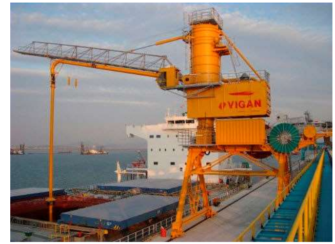
Pneumatic continuous ship unloader [Figure: Vigan]
